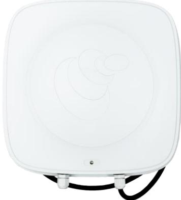
A white, square-shaped integrated RFID reader with a circular antenna on top. It has a small black cable at the bottom. |
