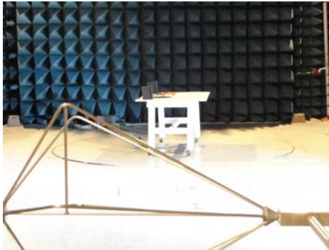
Xmtr & Rx Emissions Test Setup
