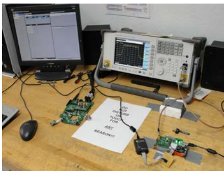
Radio Conducted Power Measurement Test Setup
