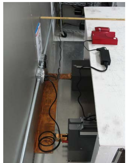
Line Conducted Test Setup
