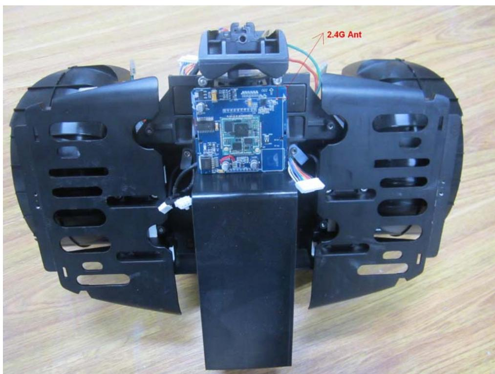
**The GSM/GPRS antenna and Wifi antenna distance from body more than 20cm.**
