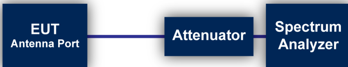
Figure 2: Direct Connection at the Antenna Port Test
