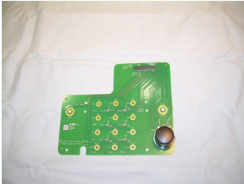
Photograph 14 – Top View of the Keypad Board
