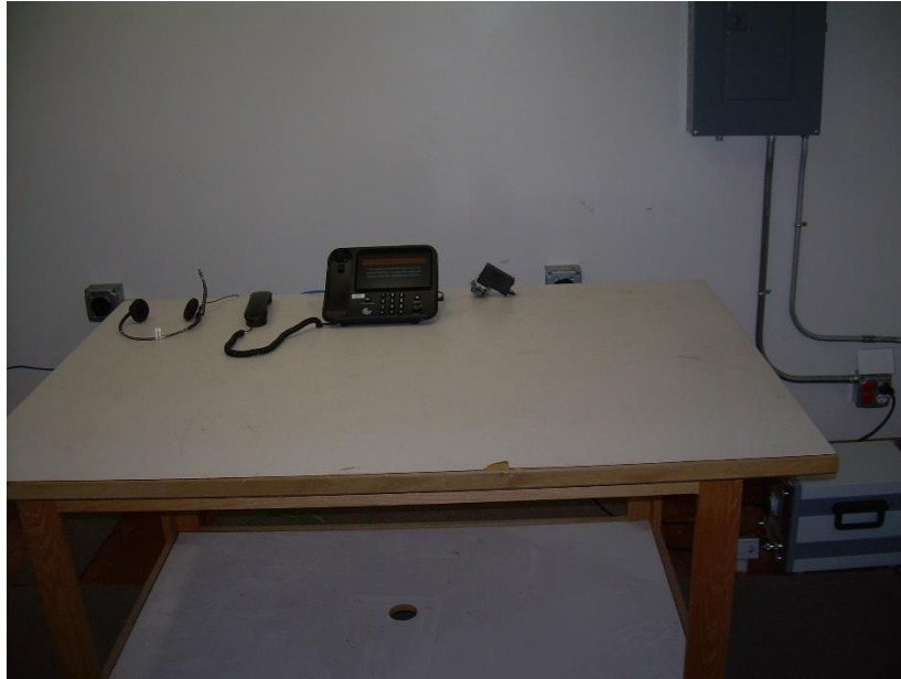
Photograph 1: Front View Conducted Emissions Worst-Case Configuration
