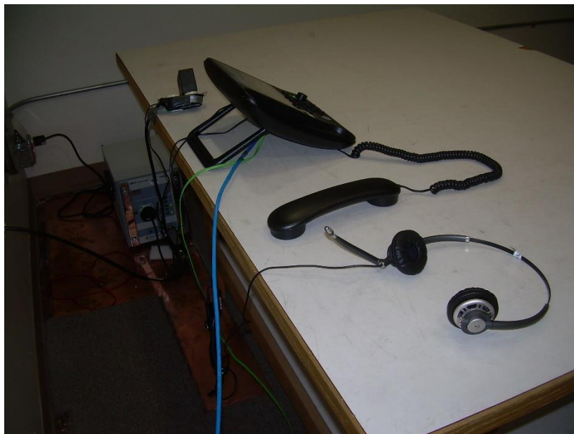
Photograph 2: Back View Conducted Emissions Worst-Case Configuration
