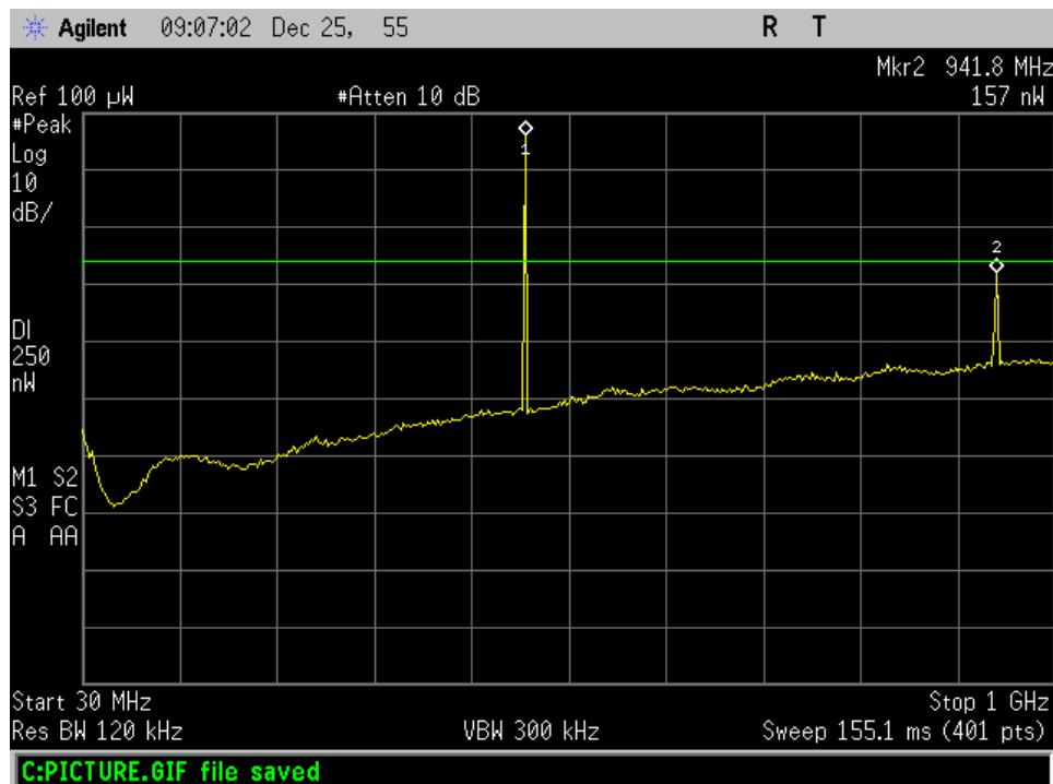
**Radiated Spurious\_ tuned freq 470.025 MHz\_30 - 1000 MHz\_4 nW limit**
