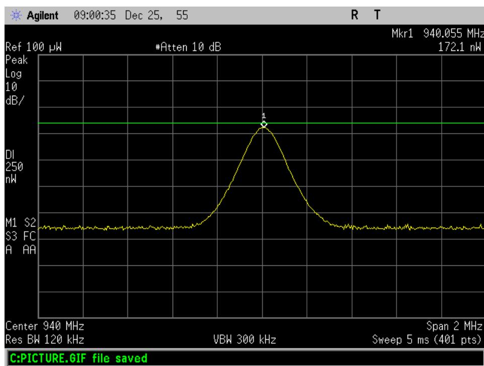
**Radiated Spurious\_ tuned freq 470.025 MHz\_30 - 1000 MHz\_250 nW limit**
