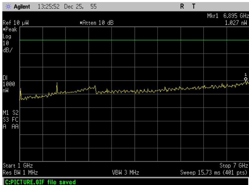
Radiated Spurious\_ tuned freq 657.025 MHz\_30 - 1000 MHz
