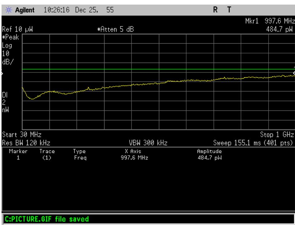
**Radiated Spurious\_ tuned freq 470.025 MHz\_1 - 7 GHz**
