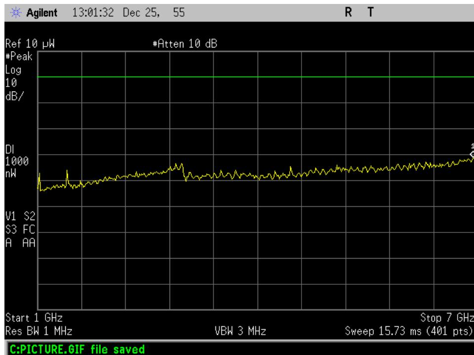
**Radiated Spurious\_ tuned freq 470.025 MHz\_2nd Harmonic 940 MHz**
