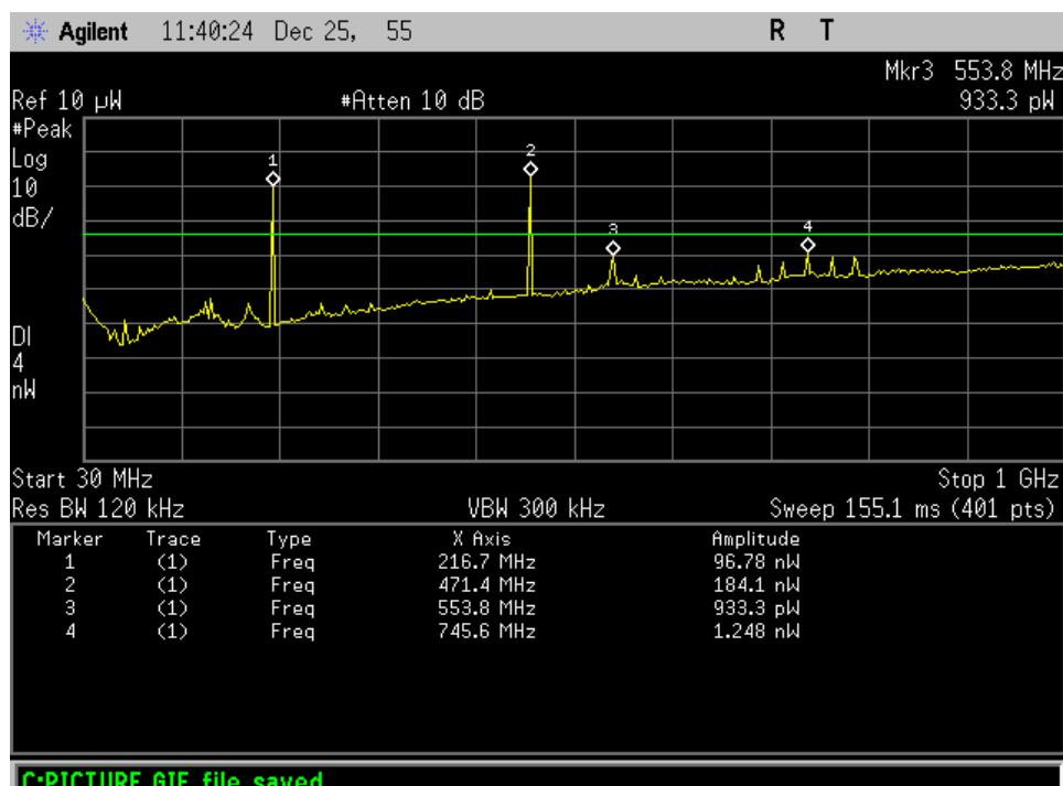
**Radiated Spurious 1 – 4 GHz\_ Beltpack = Standby\_ Base = 470.025 MHz**
