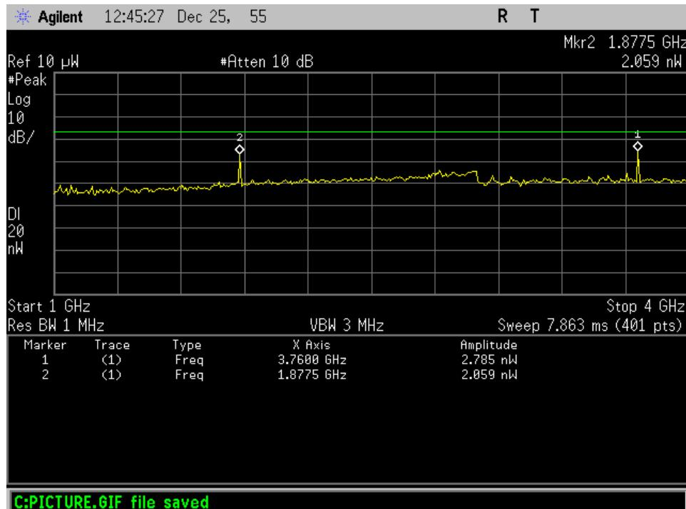
**Radiated Spurious\_30 – 1000 MHz\_ Beltpack = Standby\_ Base = 470.025 MHz**
