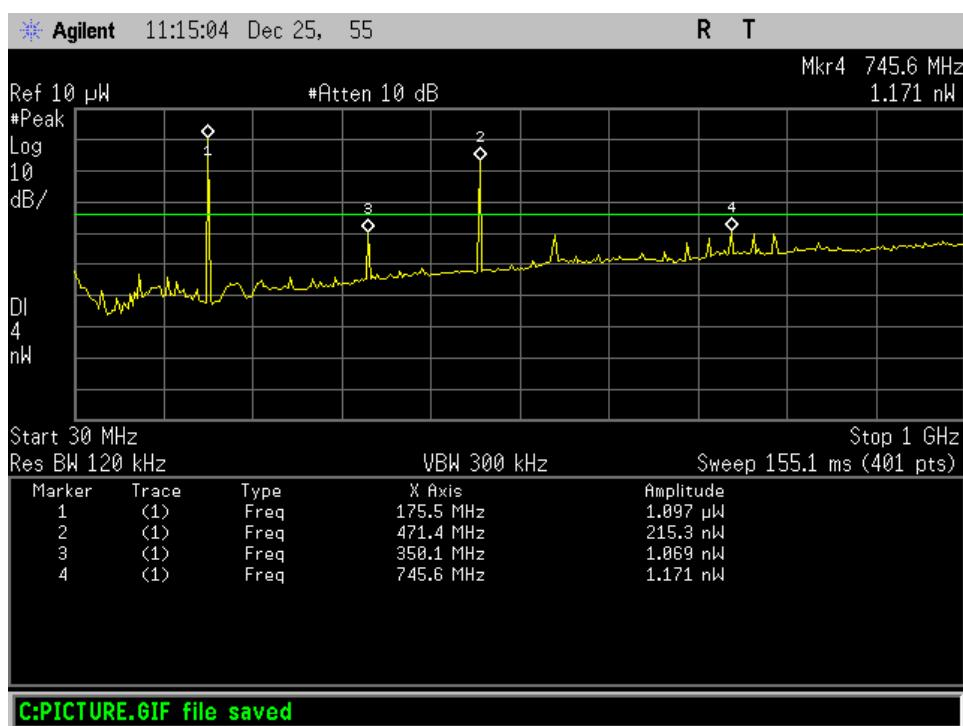
**Radiated Spurious\_1 – 4 GHz\_Beltpack = 195.025 MHz\_Base = 470.025 MHz**
