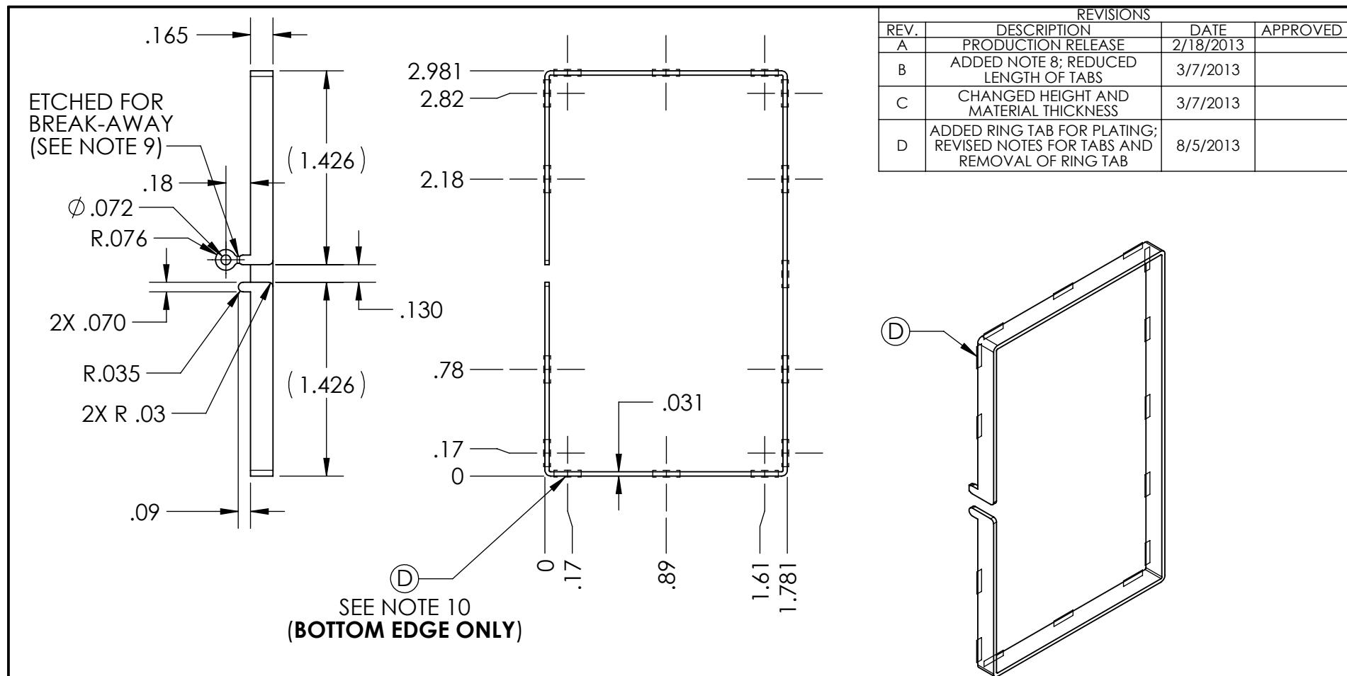
7. FINISH: SILVER PLATE PER QQ-S-365D, Type II, Grade A (**DO NOT** USE NICKEL IN THE PLATING PROCESS)
