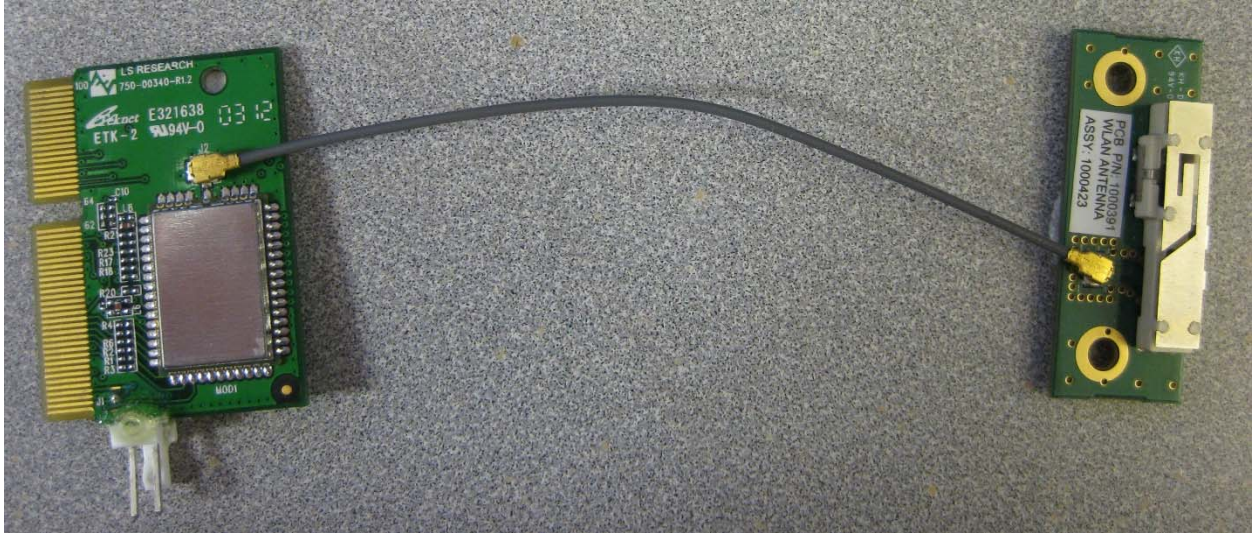
Radio module attached to board containing off module u.fl antenna connection
