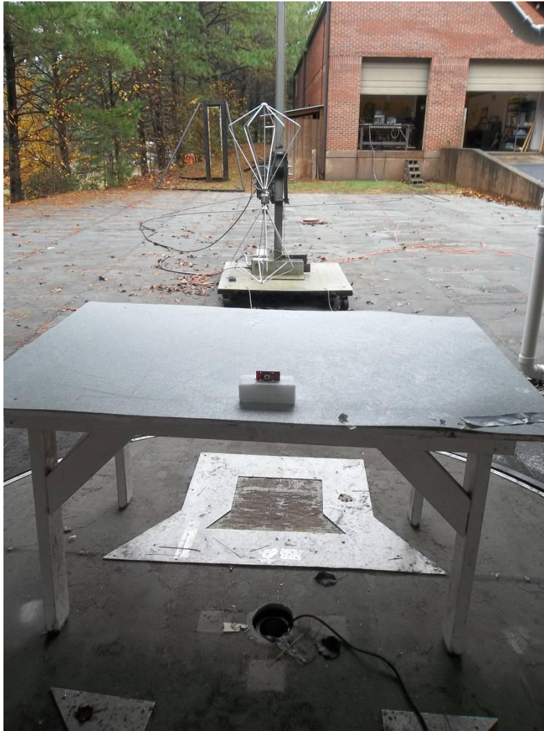
Figure 2. Test Configuration, 30 MHz - 200 MHz
