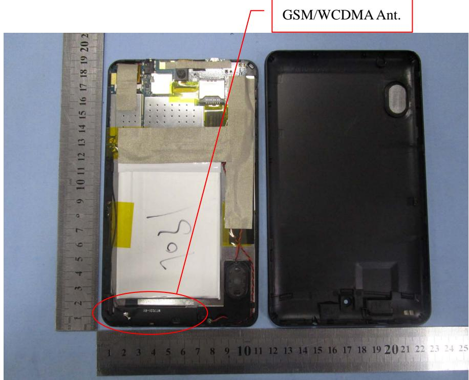
**EUT Housing and Board View 2**
