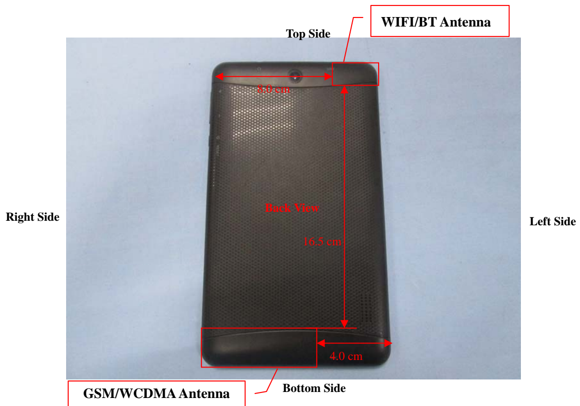
Block Diagram for EUT Antenna Position
