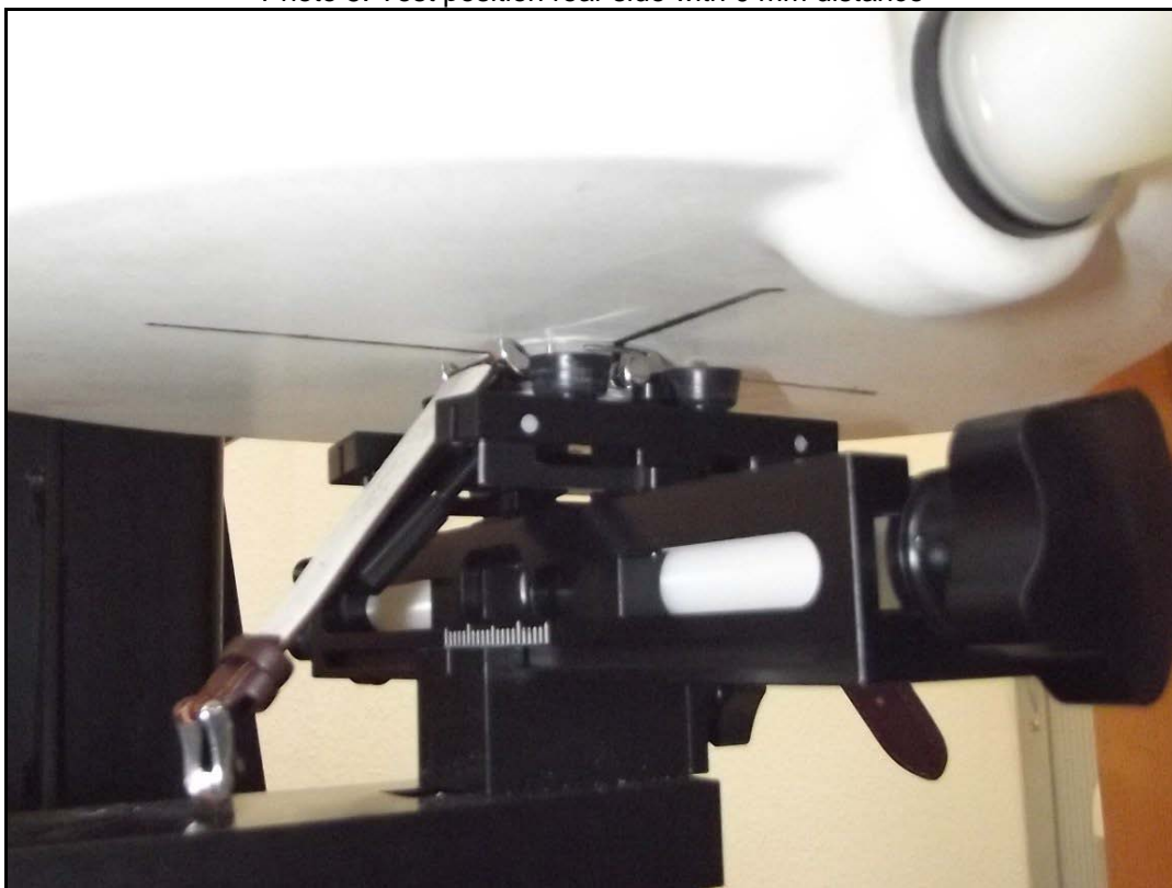
Photo 6: Test position front side with 10 mm distance
