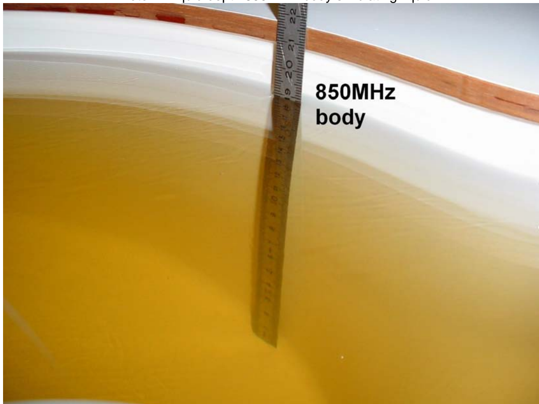
Photo 2: Liquid depth 850 MHz body simulating liquid
