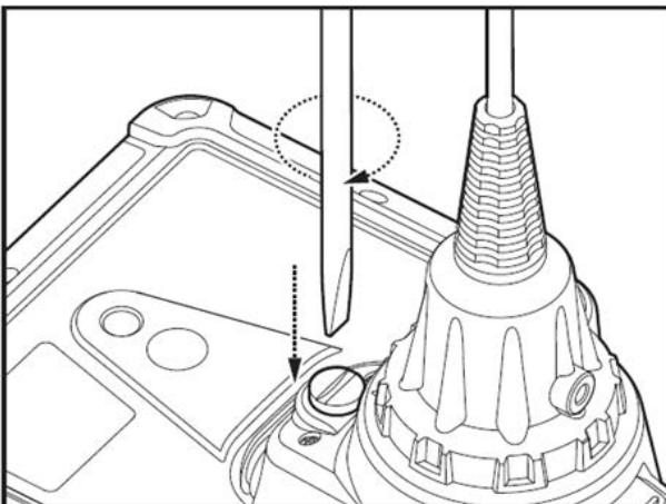
**CAUTION:** Do not remove the screw from the probe stand.
