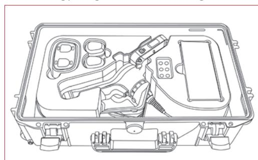
2. Do not roll the probes up too tightly (aim for a diameter of at least 15cm)
