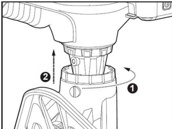
3. Align the Probe Stand's screw with the connector on the articulation probe (the long side of the stand must face inwards toward the battery release of the probe).
