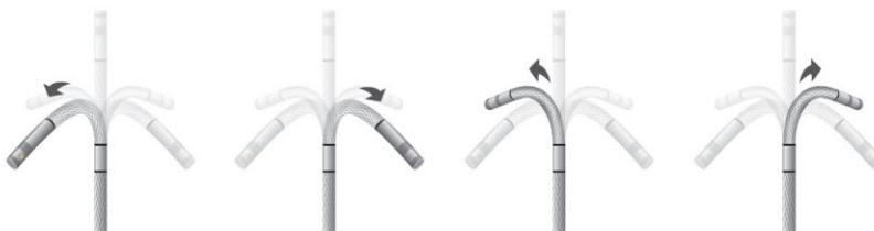
Lock mode: The articulation angle can be fixed by every joystick movement.
