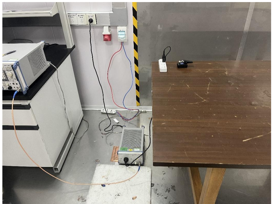
Conducted Emission Test Setup
