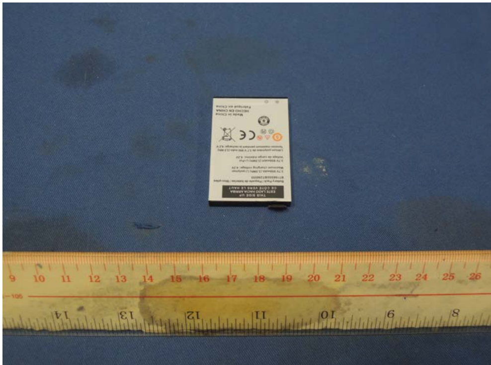
Figure 3 – 3.7VDC 950mAh Li-polymer rechargeable battery front view
