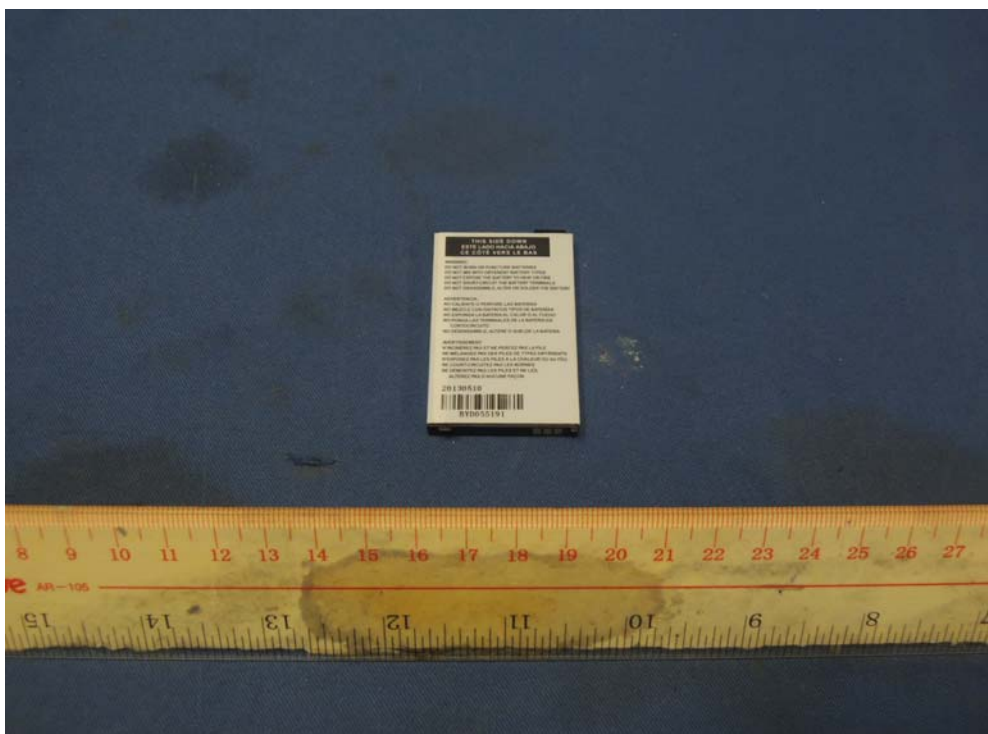
Figure 4 – 3.7VDC 950mAh Li-polymer rechargeable battery back view
