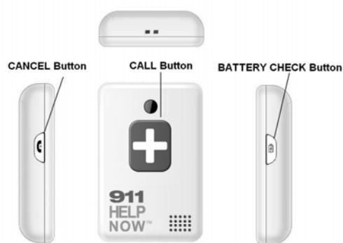
2. Press right side battery check button. Front LED light will light green. If the LED Light is not on, recheck position of the batteries and repeat Until green light is on.
