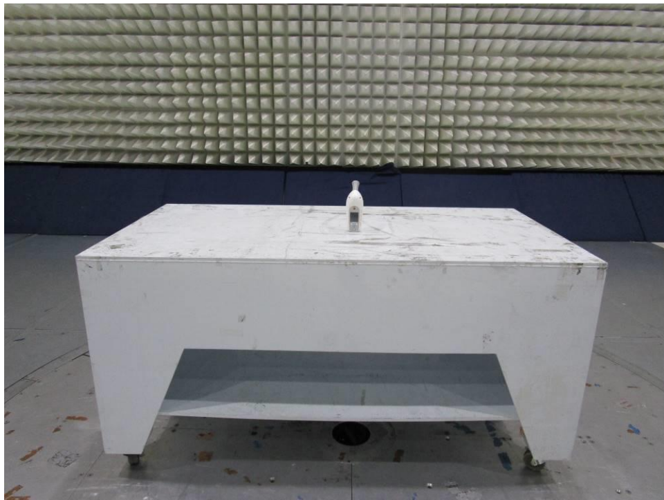
Electromagnetic Radiated Disturbance Setup Photograph
