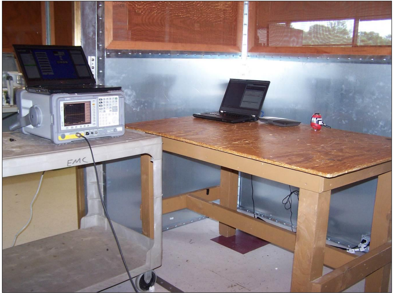
Photograph 3. Conducted Emissions, 15.207(a), Test Setup
