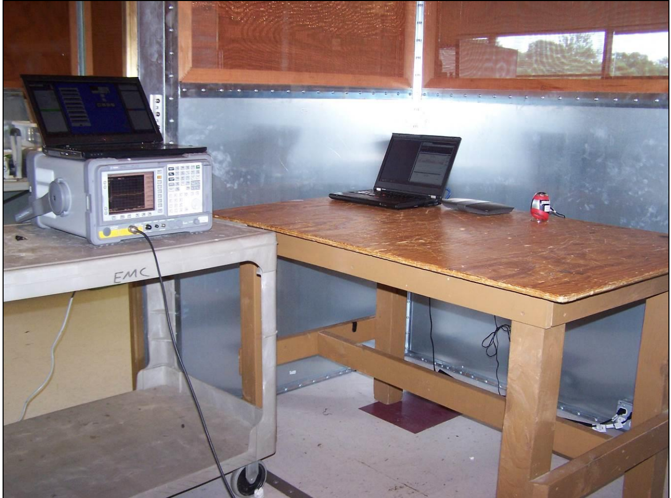
Photograph 4. Conducted Emissions, 15.207(a), Test Setup
