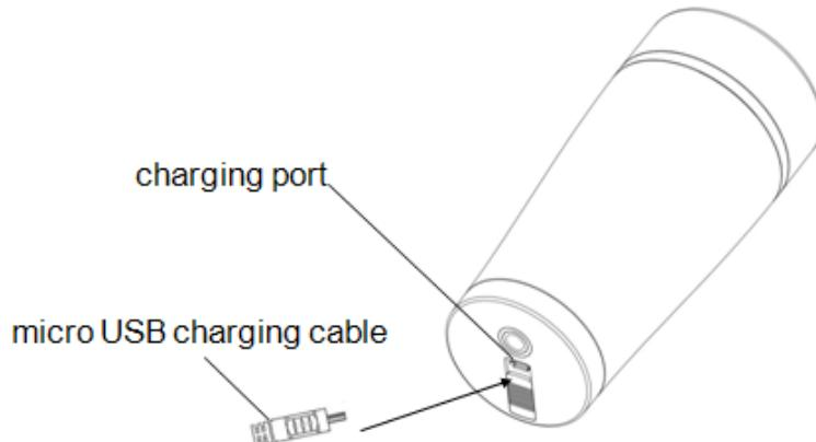
Finished charging: When LED flashes from slow to stable,Efee is fully charged.
