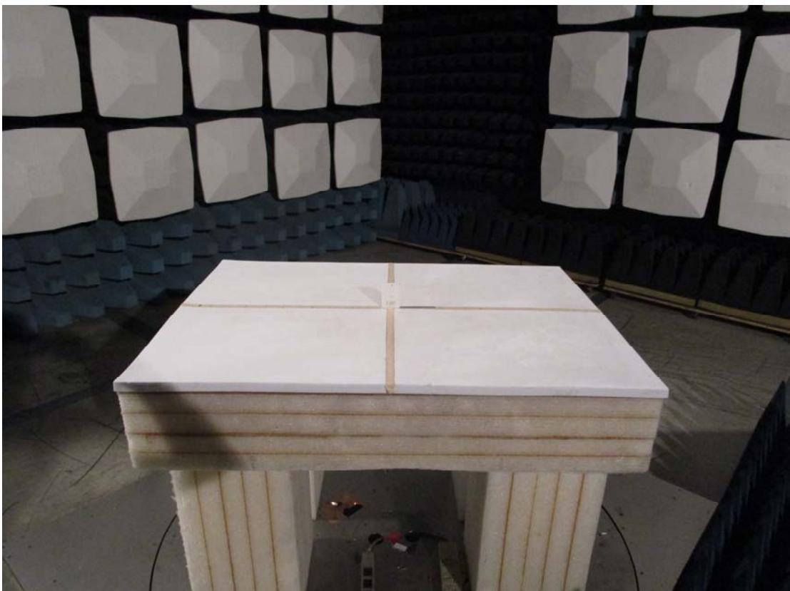
**RADIATED RF MEASUREMENT SETUP****Below 1GHz**
