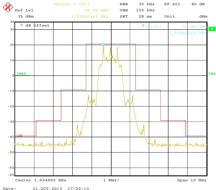
**High Channel (Unwanted Emission inside the Sub-band)**
