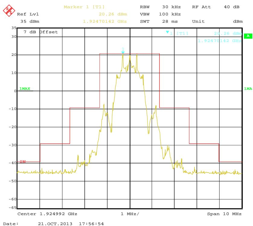
**High Channel (Unwanted Emission inside the Sub-band)**
