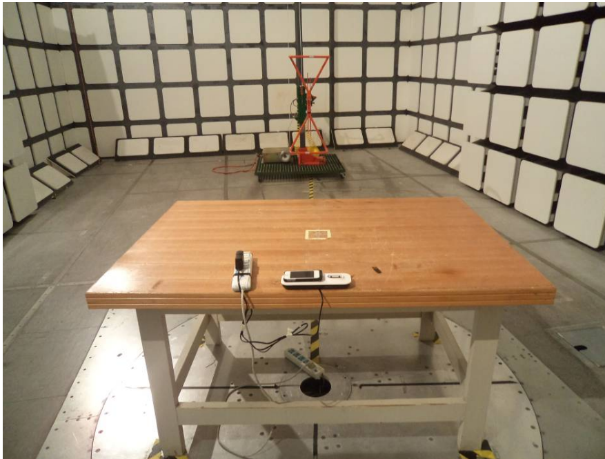
Radiated Emission – Rear View (30 MHz to 1 GHz)
