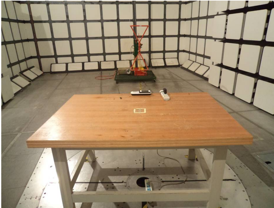
Radiated Emission – Front View (30 MHz to 1 GHz)
