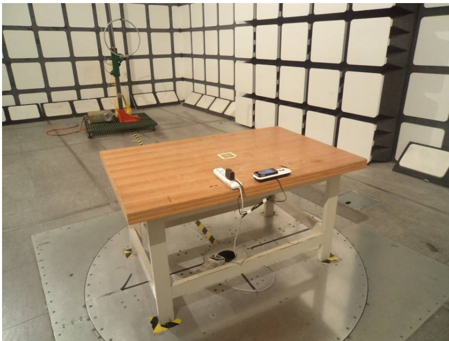
Radiated Emission – Rear View (9 kHz to 30 MHz)
