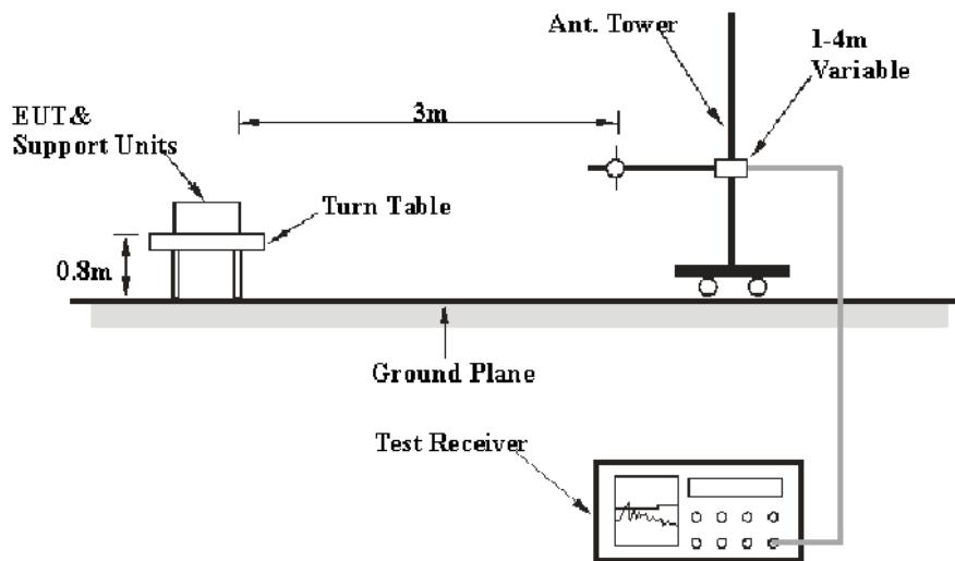
The radiated emission and out of band emission tests were performed in the 3 meters chamber test site, using the setup accordance with the ANSI C63.4-2009. The specification used was the FCC 15.209 and 15.205 limits.
