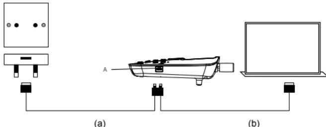
1. Plug the USB cable into socket (A) on the side of the base.
