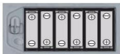
※When installing batteries, please start from cathode end first.
