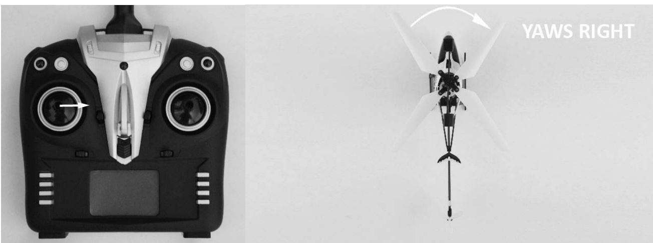
The rudder trim lever (located immediately below the left-hand stick for Mode 2) can be used to help keep the nose of the helicopter from turning (yawing) to the left or right when 'hovering' and without any left-hand stick/rudder control input. For example, if the nose of the helicopter turns to the right when hovering add left rudder trim by pressing the lever to the left until the nose of the helicopter stays as close to 'straight' as possible with no further input.
