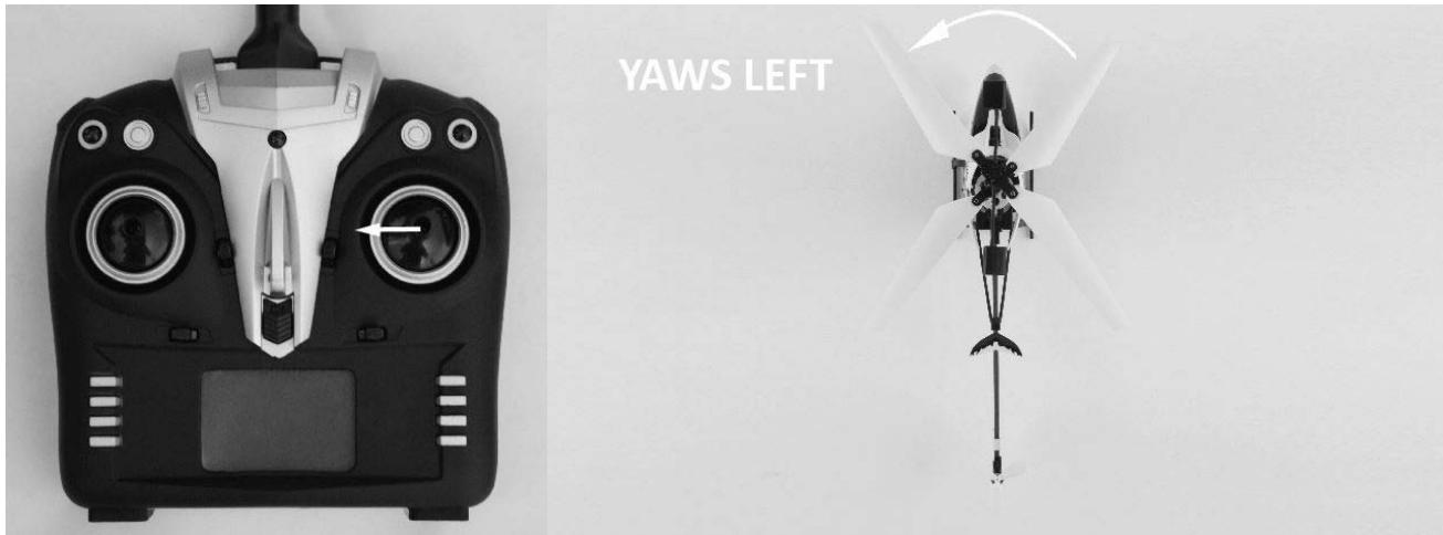
Moving the stick to the right will turn (yaw) the nose of the helicopter to the right about the vertical axis. This is accomplished by increasing the speed of the lower rotor blades and decreasing the speed of the upper rotor blades.
