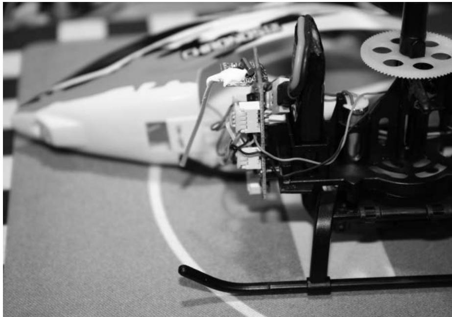
Re-install the canopy by carefully sliding it over the control unit and battery while also aligning the mounting 'slots' inside the canopy with the mounting 'tabs' located on the left and right sides of the frame. Then carefully slip the left and right ends of the canopy over the mounts by aligning them with the mounting holes.
