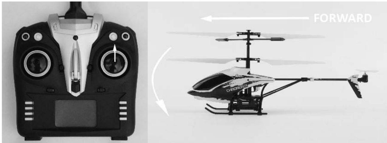
Pulling the stick backward will cause the tail motor and rotor blade/propeller to spin in the opposite direction in order to pitch the tail of the helicopter downward so it can be flown backward.
