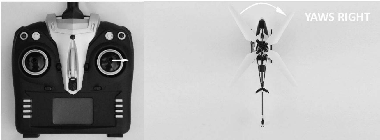
The rudder trim lever (located immediately below the right-hand stick for Mode 4) can be used to help keep the nose of the helicopter from turning (yawing) to the left or right when 'hovering' and without any right-hand stick/rudder control input. For example, if the nose of the helicopter turns to the right when hovering add left rudder trim by pressing the lever to the left until the nose of the helicopter stays as close to 'straight' as possible with no further input.
