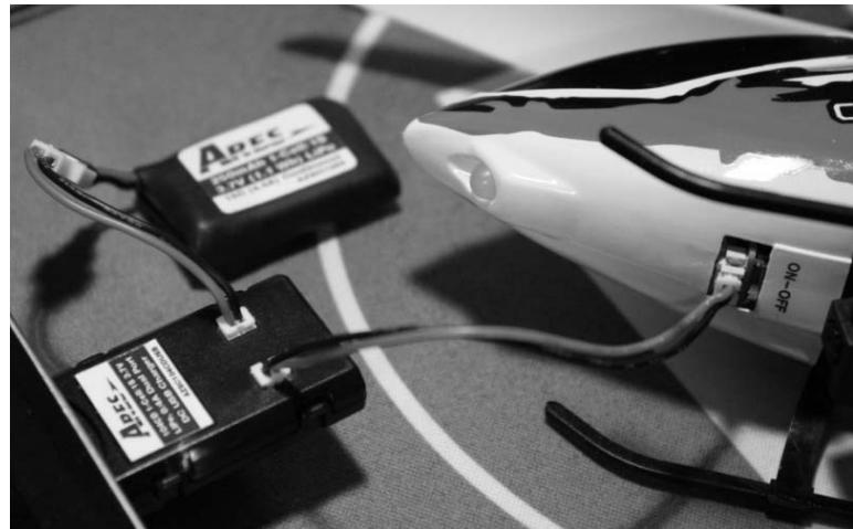
**NOTE: The reference photos show the dual port DC USB charger charging a spare LiPo battery (AZSH1355; sold separately) while charging the battery installed in the helicopter at the same time. You can also purchase an additional Micro A Female Connector to Ultra-Micro Male Connector Adapter Lead (AZSH1354) to charge two batteries that are not installed in the helicopter at the same time.**
