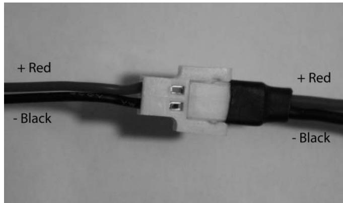
Also, although the 'Micro A' connectors are 'keyed' to minimize the risk of a reverse polarity connection, if you force them it is possible to make connection with incorrect/reversed polarity potentially causing damage to the control unit and/or battery. When the connectors are properly aligned for correct polarity, connecting them should require only a minimal amount of pressure to achieve the light 'click' that indicates secure connection.
