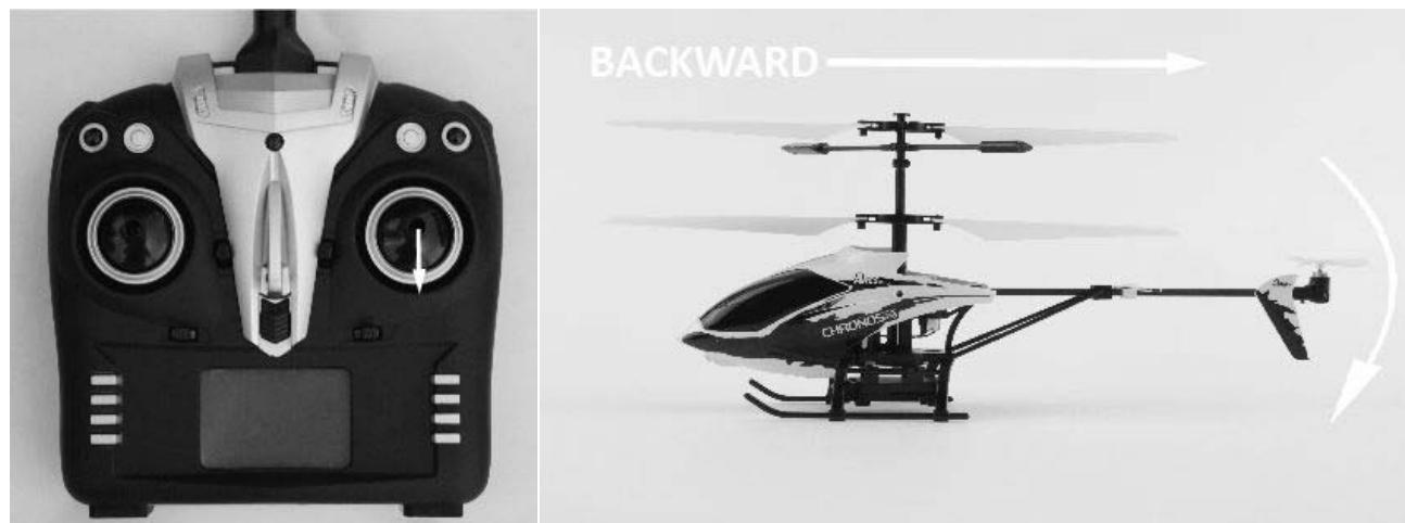
The elevator trim lever is located immediately to the left of the right-hand stick. **And although the position of the elevator trim can be changed, because the Chronos CX 100 is equipped with a motor for elevator control the trim has no actual effect on the helicopter.**
