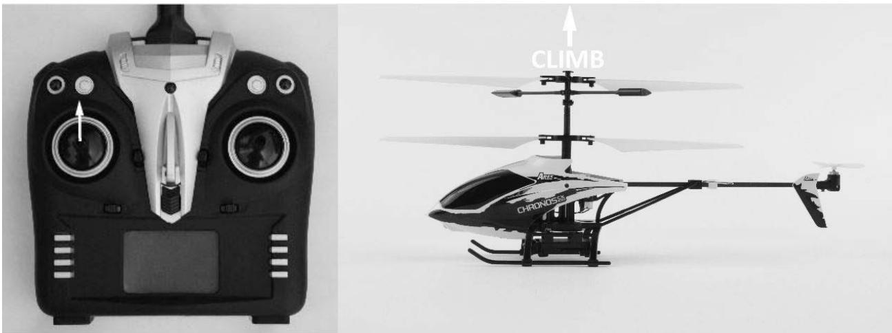
Decreasing the RPMs/speed of the rotor blades by lowering the left-hand stick will cause the model to descend.
