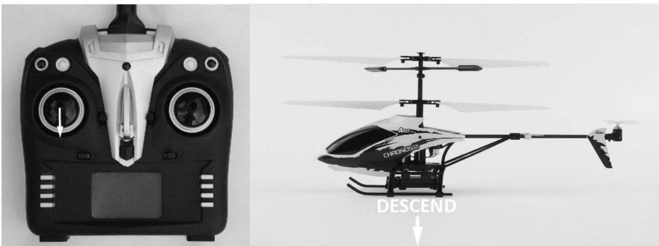
After lifting the model off the ground you can 'hover' by carefully moving the left-hand stick up and down slightly as needed so the model will maintain altitude without climbing or descending.
