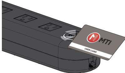
**1b** From an Alarming state, place the User Key over the RFID icon to silence the alarm. Then hold down the User Key for 5 seconds to return back to the disarmed state. LED will be flashing white.
