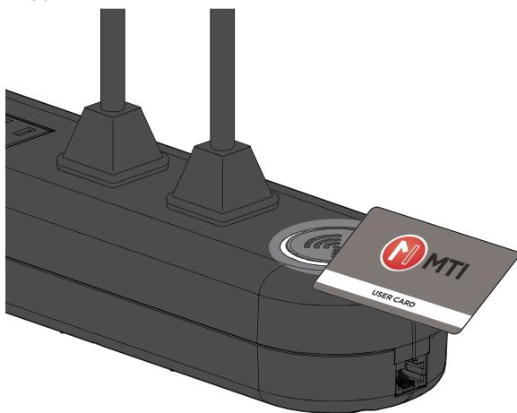
**3** If any cable becomes unplugged, the system will alarm. LED will flash red/white. The Remote Access Module will show a corresponding red LED for that socket port.
