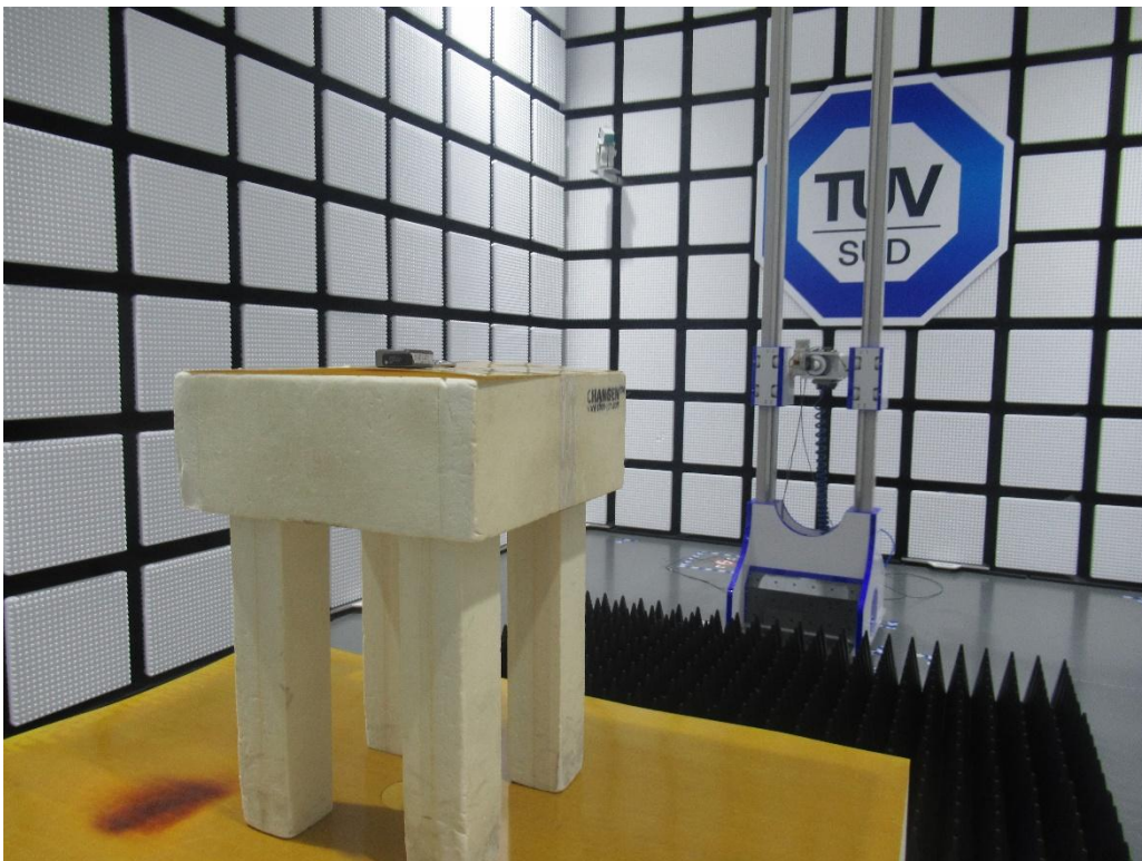
Radiated Emission Test above 18 GHz
