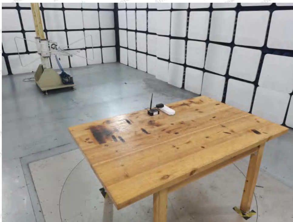
Photo of Radiation Emission Test
