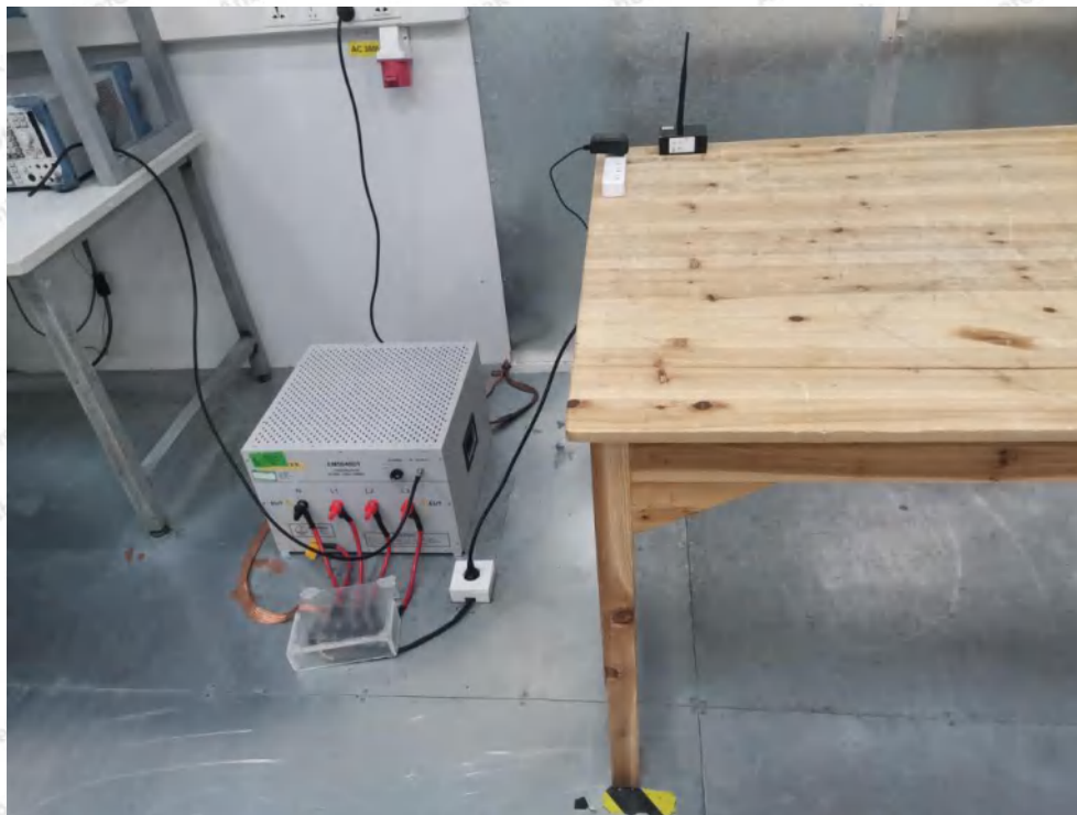
Photo of Conducted Emission Measurement
