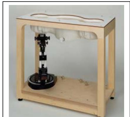
The bottom plate contains three pair of bolts for locking the device holder. The device holder positions are adjusted to the standard measurement positions in the three sections. A white cover is provided to tap the phantom during off-periods to prevent water evaporation and changes in the liquid parameters. On the phantom top, three reference markers are provided to identify the phantom position with respect to the robot.
