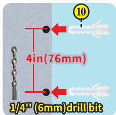
1. Punch holes in the wall to plug the expansion plug
