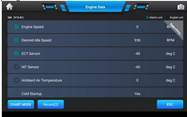
Press the button **[CHART MODE]** to show the data in graphic or press the button **[TEXT]** to show the data in text.
