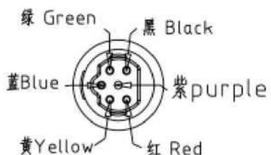
The S90 lock has a 6PIN connector, which allows for a lot of expandable features through the connector, including Solar panel charging, EBIKE integration, Type-C charging, etc.
