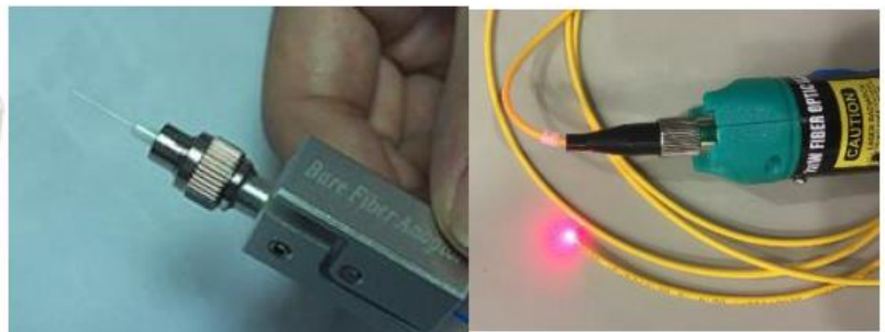
Test steps: insert optical fiber / test on-off
