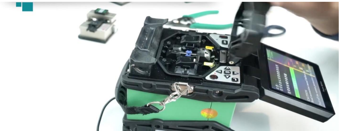
12. Fix the cable and pigtail into the splicing box of single core optical fiber fusion splicer
