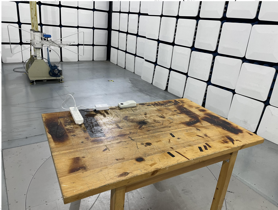
Photo of Radiation Emission Test (below 1GHz)
