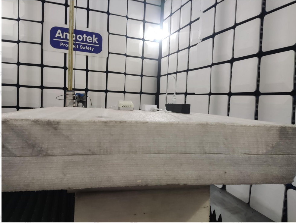
Photo of Radiation Emission Test (above 1GHz)
