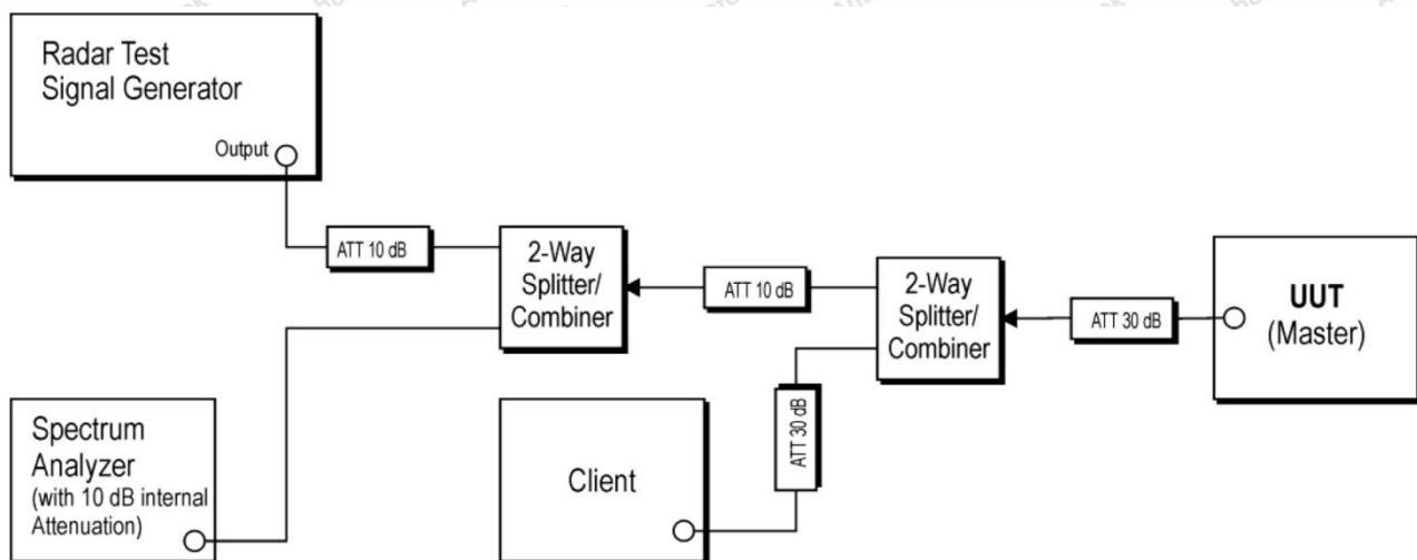
Radar Test Waveforms are injected into the Master.
