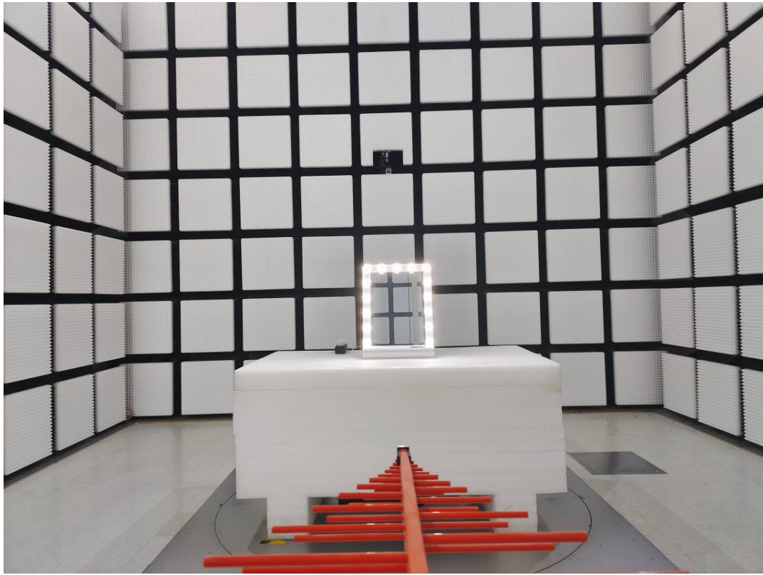
Radiated Emission Above 1GHz View
