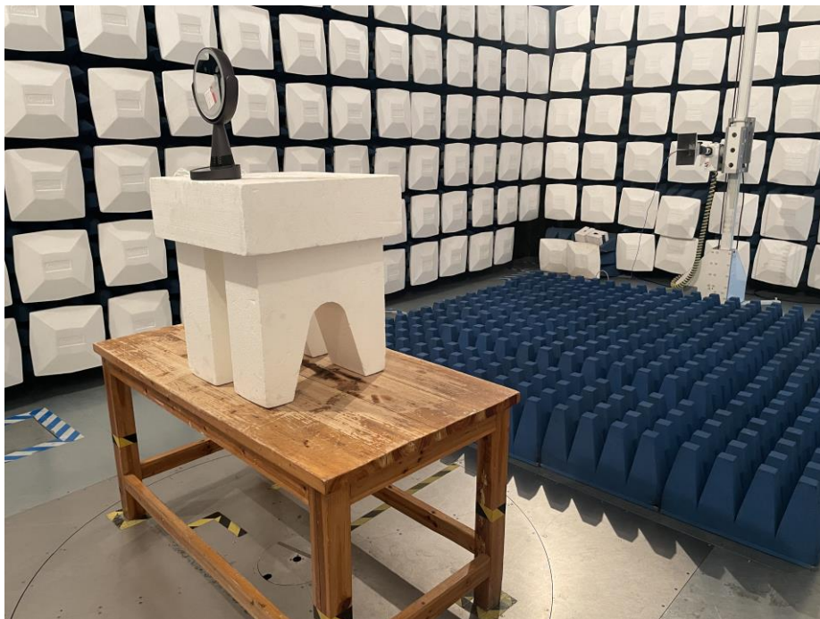
Test Setup For Radiated Emission (Above 1GHz)
