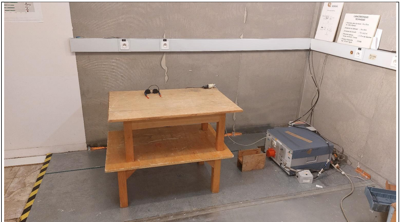
Test set up of conducted emission on power supply
