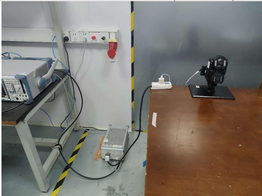
Conducted Emissions at Mains Terminals (150 kHz-30MHz)
