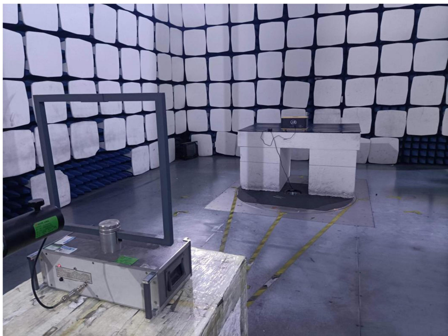
Radiation Emission Test Setup (Below 30MHz)
