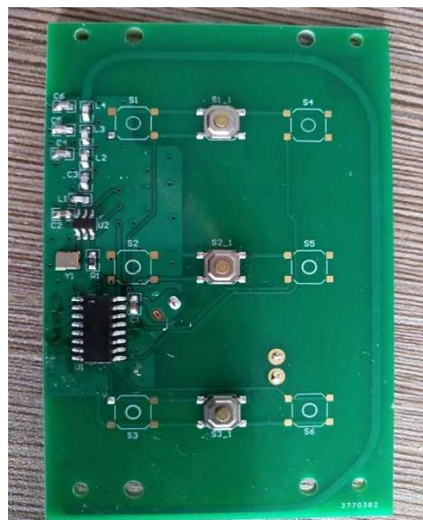
Antenna transmission frequency: 433.92MHz
