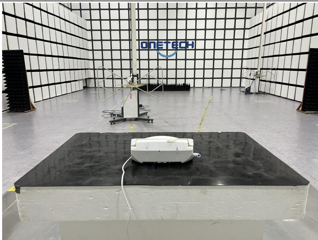
**- Radiated Emission Test (Above 1 GHz)**
