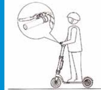
6. Apply pressure to the brake lever to slow down or stop.
