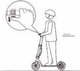
5. Continuously press the throttle to speed up.
