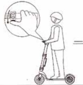
4. Press the THROTTLE slightly with your right hand to start and rotate the handlebars to turn.
