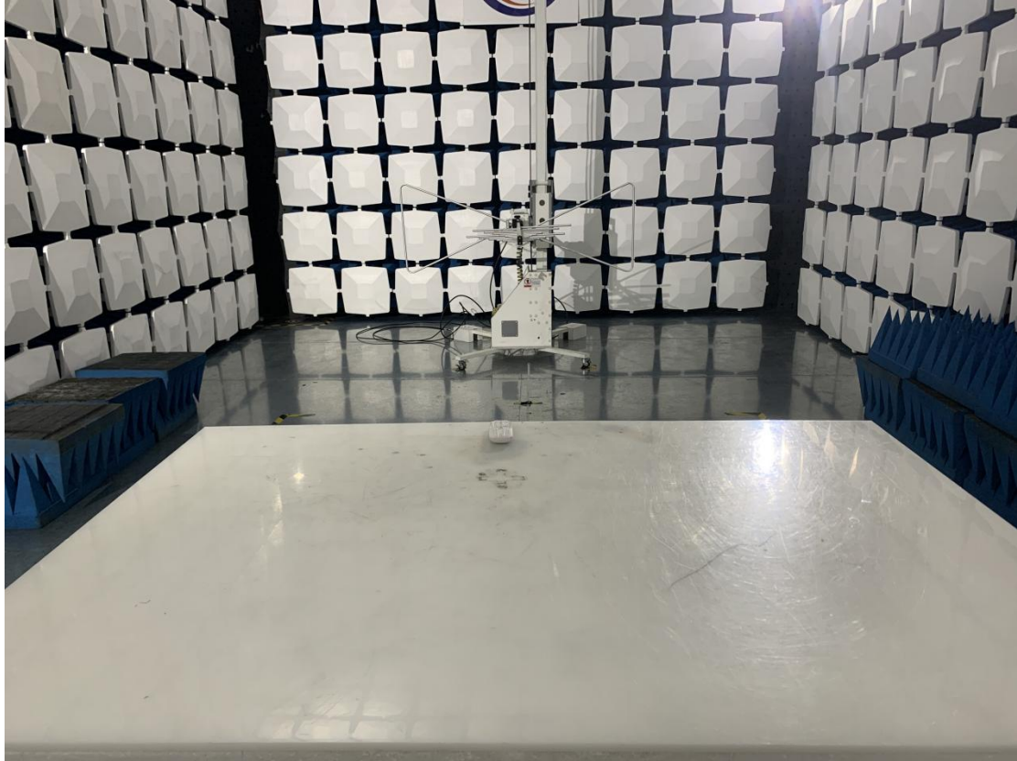
Above 1GHz for radiated emission test setup
