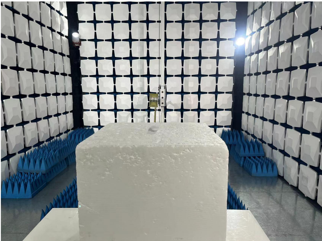
Above 1GHz for radiated emission test setup
