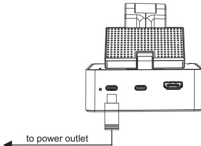
When the battery is full, you can remove the power cord and power it directly through the battery. Next, press and hold the power button for one second. Boot-up time is approximately 60 seconds.
